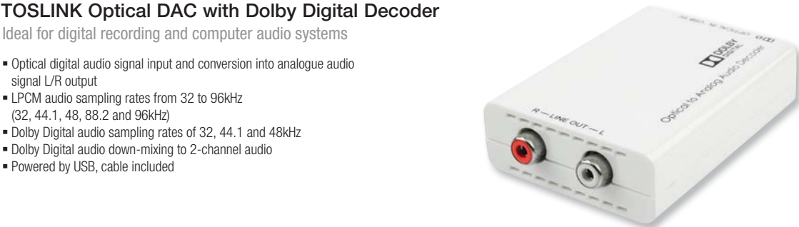
TOSLINK Optical DAC with Dolby Digital Decoder
