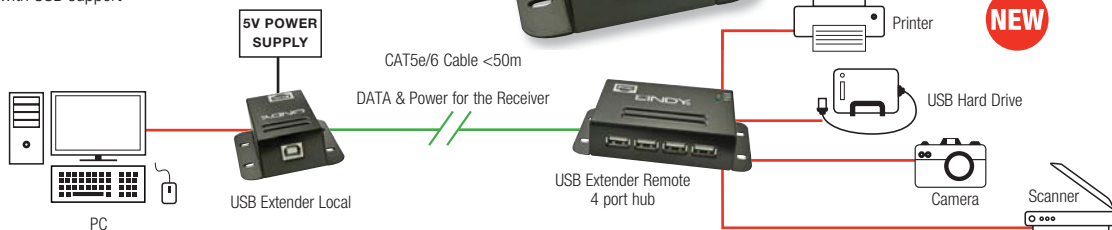
50m USB 2.0 4 Port CAT.5/6 Extender with Power Over CAT.5/6
