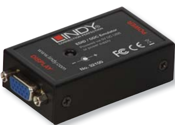
EDID/DDC Emulator Programmer for VGA/DVI & HDMI Displays 32100
